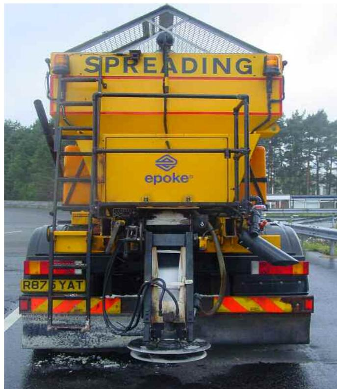
Figure 2. A typical Epoke spreader during the TRL performance trial
