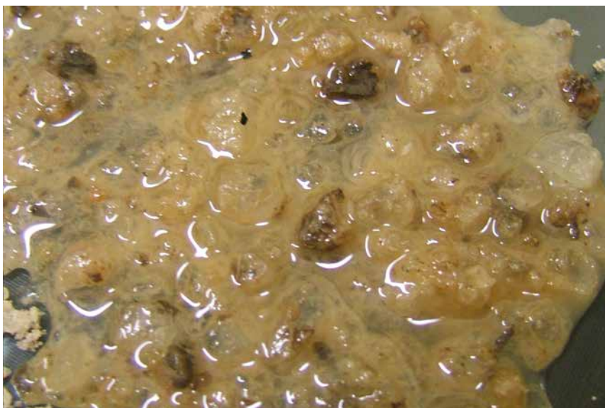
Figure 5.4.2 - Pre-wetted salt (dry salt to brine ratio 70:30 by weight)
