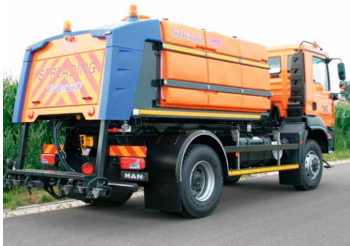
Figure 5.6.2 - A DLA spreader with spray nozzles for treating three lanes
