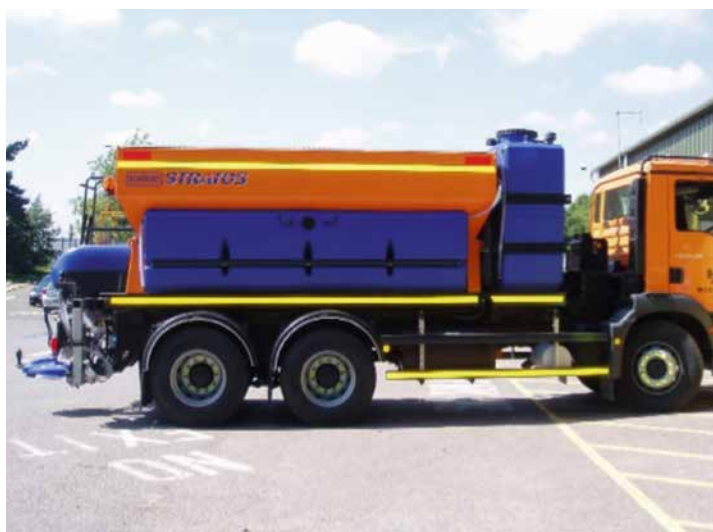
Figure 5.6.3 – A combination spreader that can deliver DLA only treatments as well as pre-wetted treatments
